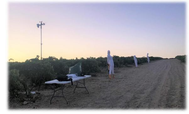
4 trials in grape vine were conducted comparing operator exposure (pilot and auxiliary activities<sup>1</sup>) and bystander and resident drift exposure during UASS application vs. conventional application (EFSA OREX Guide<sup>2</sup>) M&L), purge, battery changes and maintenance and cleaning activities <sup>2</sup> doi: 10.2903/j.efsa.2022.7032
